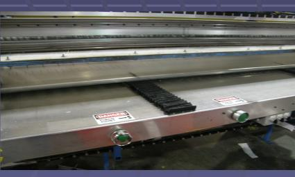
• Accordion safety guard on the forward position on HMB #3.
