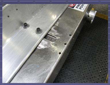
HMB #2 missing accordion safety guard on right side.
