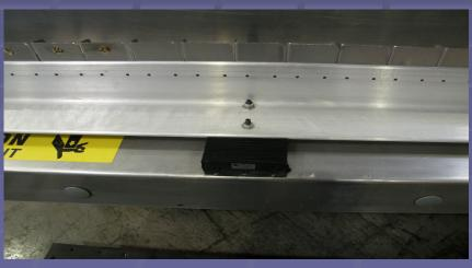
HMB #1 with correct accordion safety guards.
